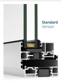
Thermally broken window that allows for both side hung and top hung outward openings. This solution, with a thermal break zone of 32 mm and a transmittance Uw from  $0.9 \text{ W/m}^2\text{K}$ , has the British security certification PAS 24, being especially suitable for this market.
